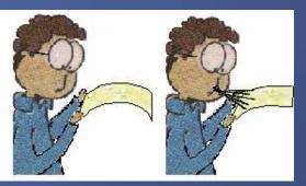
Bernoulli's principle – as speed of a fluid increases, the pressure inside the fluid decreases
