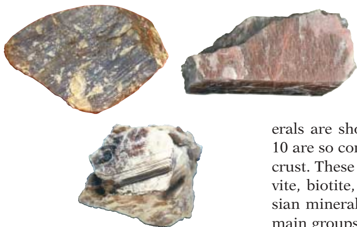
Figure 1 ▶ Plagioclase feldspar (left), muscovite mica (center), and orthoclase feldspar (right) are 3 of the 20 common rock-forming minerals.
