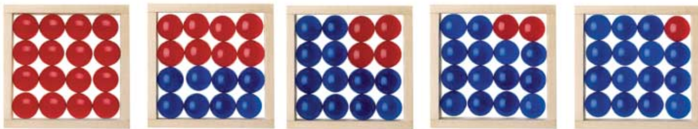
Figure 4 ► After each half-life, one-half of the parent isotope is converted into a daughter isotope. After four half-lives, only 1/16 of the parent isotope remains.
