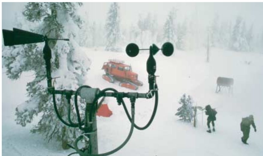
Figure 1 ▶ Weather instruments, such as these at Elk Mountain weather research facility in Wyoming, indicate wind speed and direction.
