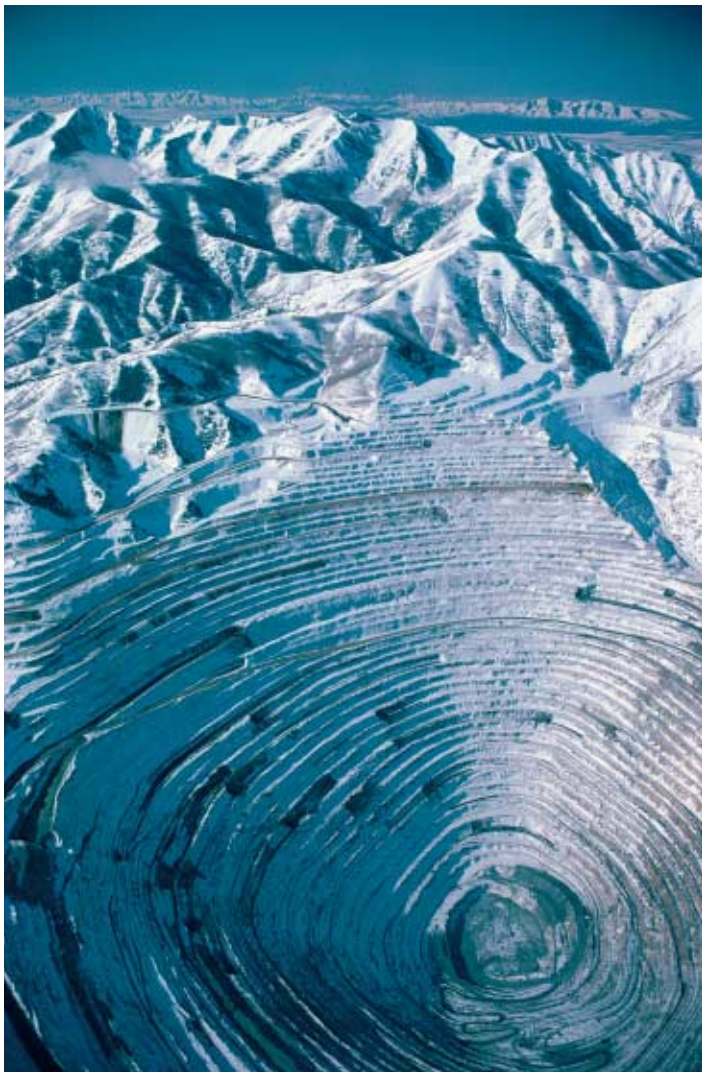
Figure 3 ▶ With a rim diameter of 4 km and a depth of almost 1 km, the Bingham Canyon Mine in Utah is the largest copper mine in the world.
