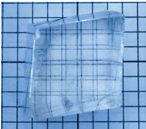
Figure 5 ▶ Some forms of the mineral calcite exhibit double refraction when light rays enter the crystal and split.
