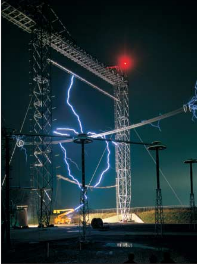
Figure 5 ▶ An outdoor ultrahigh-voltage laboratory generates artificial lightning to test its affects on electrical utility equipment. Research has led to the development of equipment that suffers less damage from lightning.
