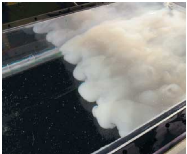
This simulated turbidity current was created in a laboratory. The density of the sediment-filled water causes it to move downhill like a landslide does.
