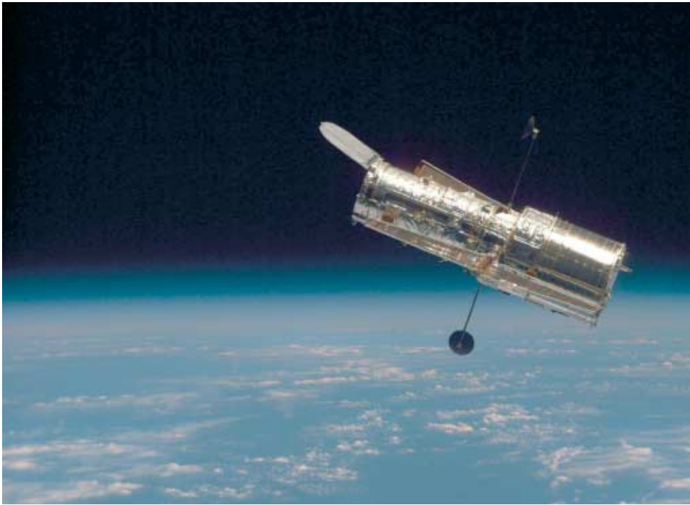
Figure 7 ▶ The Hubble Space Telescope is in orbit around Earth, where the telescope can detect visible and nonvisible electromagnetic radiation without the obstruction of Earth's atmosphere.
