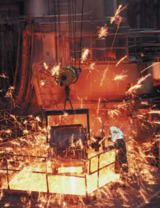
Figure 6 ▶ The steel that is being smelted in this steel mill in Iowa is a solution of iron, carbon, and various other metals such as nickel, chromium, and manganese.
