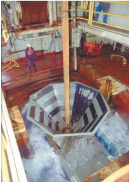
Figure 2 ▶ Reentry cones (above) are used so that core samples can later be taken from the same place on the ocean floor. Scientists aboard the research ship JOIDES Resolution (right) perform scientific studies of the ocean floor.
