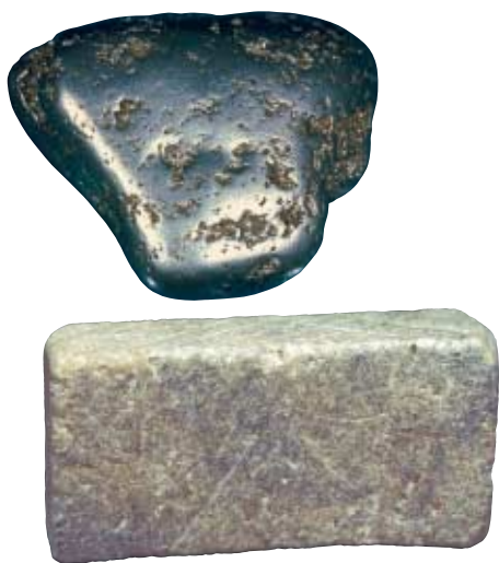
Figure 2 ▶ All minerals have either a metallic luster, as platinum does (top), or a nonmetallic luster, as talc does (bottom).
