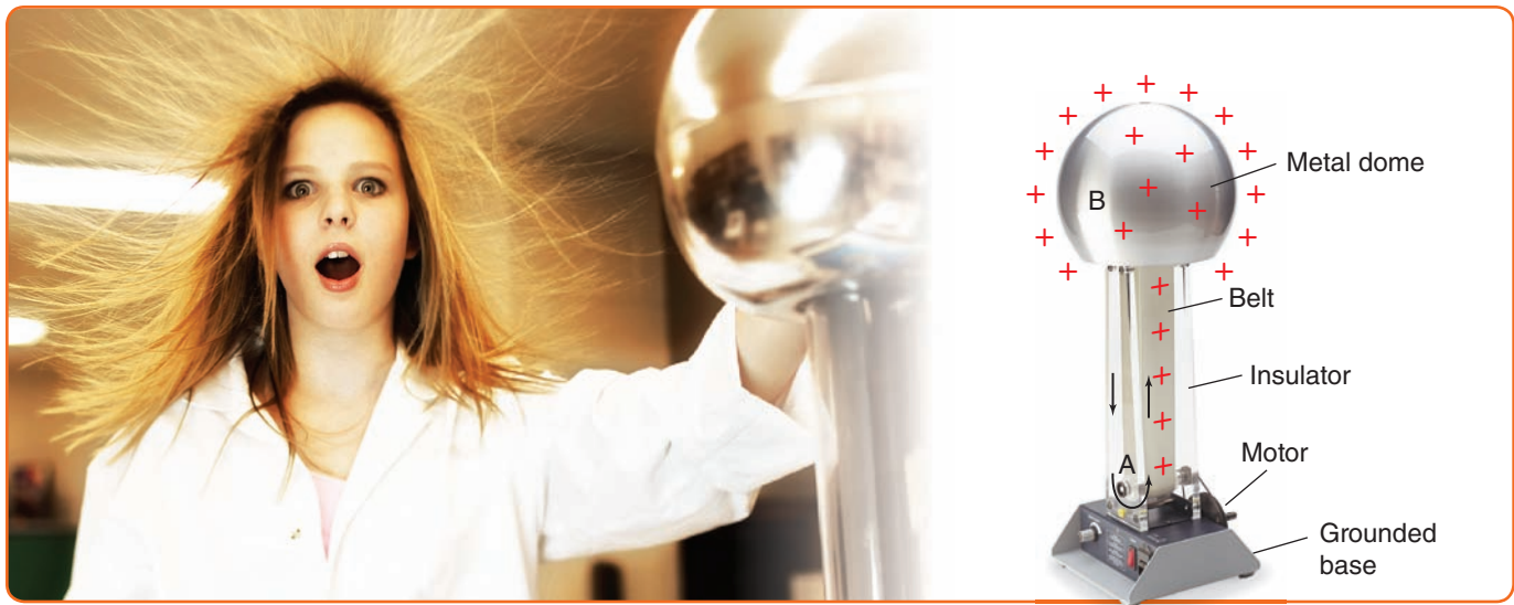
Figure 7 Robert Van de Graaff devised his generator in the 1930s to aid in the study of particle acceleration and the study of the structure of the atom. When a person touches the generator, the charges on the person's hairs repel each other, causing the hairs to align with the electric field of the metal dome.
