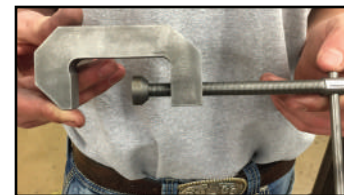
Pictured, left, is Clayton Stevens shown with his class project. He used the mill and lathe to manufacture a C-Clamp.
