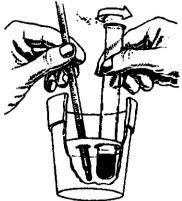
9. When the temperature of the water has stopped increasing, Record this temperature. (T<sub>2</sub>)
