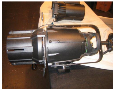
Figure 42: Ellipsoidal without the barrel
