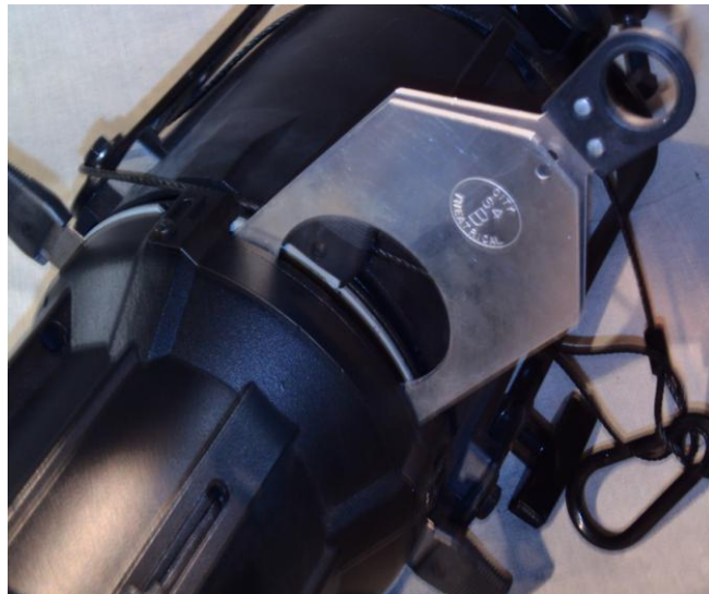
Figure 31: Gel frame half in a ellipsoidal
