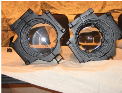
Figure 40: A 50° and a 36° barrel side by side.
