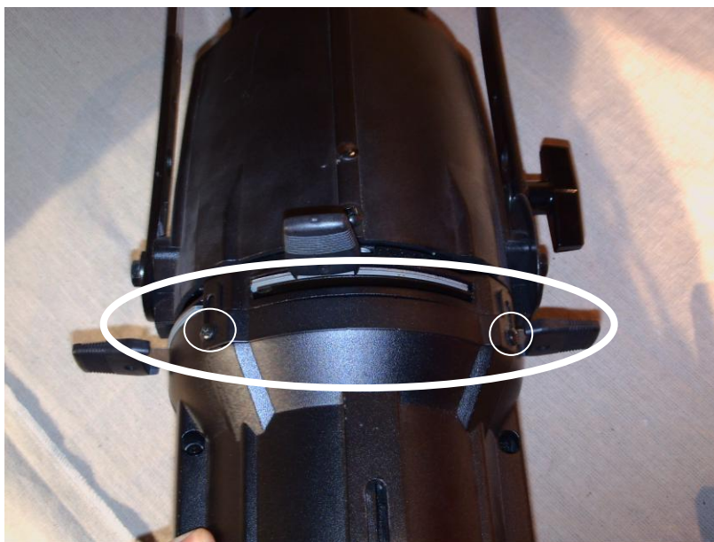
Figure 36: Cover and screws (still on)
