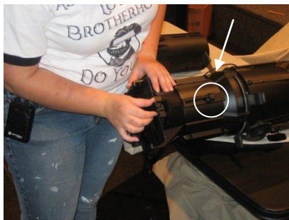
Figure 41: knob to release the barrel
