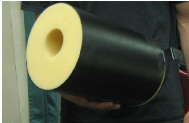
Figure 60: Fog Silencer Nozzle
