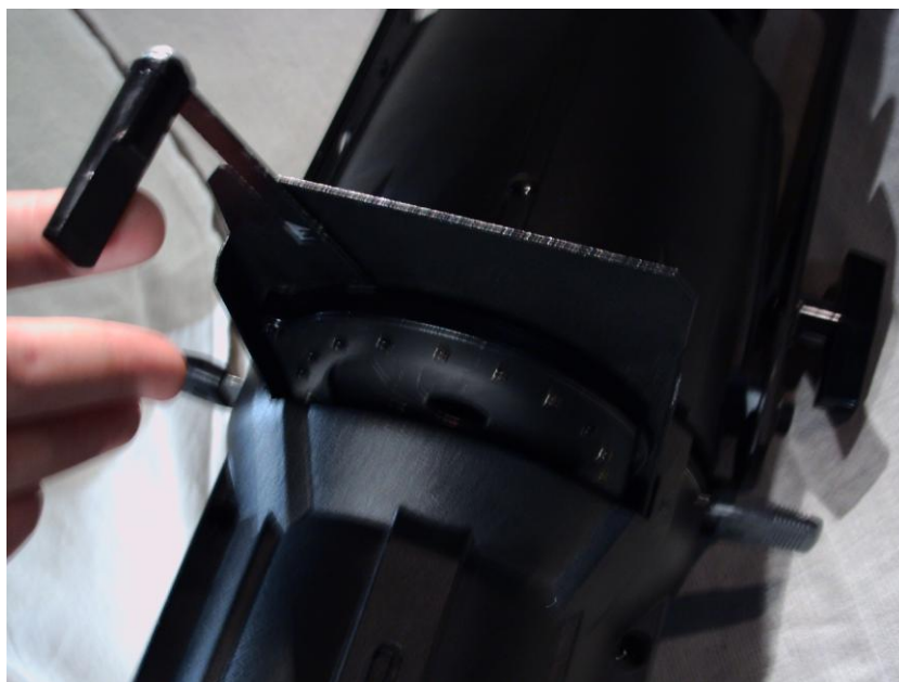
Figure 38: Iris half in the ellipsoidal
