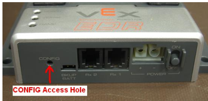
ii. VEXnet Cortex CONFIG Switch Access Hole
