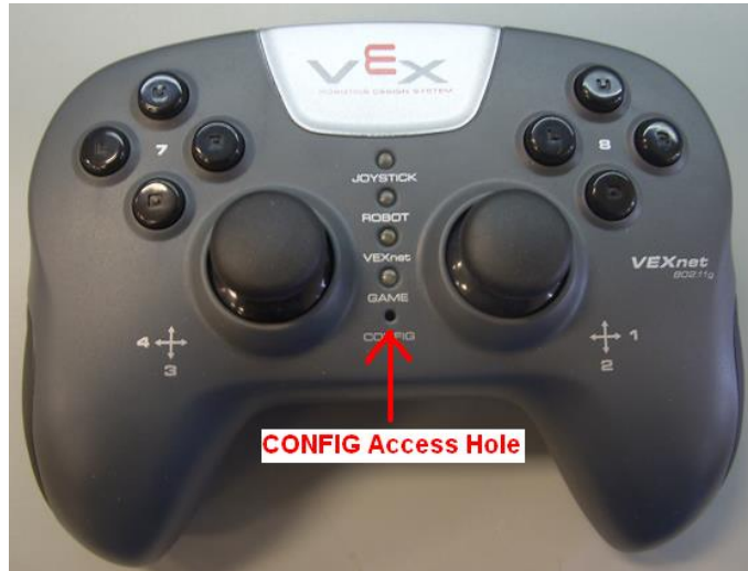
i. VEXnet Joystick CONFIG Switch Access Hole
