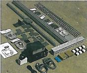
Kit includes the full gantry except for the driveshaft, which you fabricate from 3/4" cold roll round bar.
