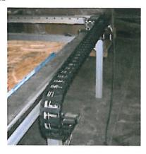
available to help you isolate your plasma torch cable from your electronics cables. Cable carriers come with lengths for both X and Y axes.
