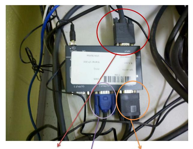
The VGA spliter has one grey cable that goes to the computer. The big black cord from the ELMO is on the other side. The final cord is the monitor cable from your monitor
