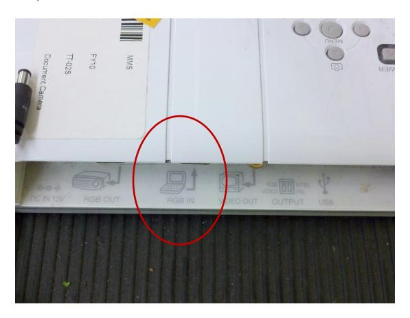
The next big black VGA cable will plug in here. It will attach to the VGA spliter (shown in the next picture).
