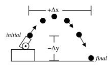
In this example, the object has a positive x-displacement (because it moved to the right) and a negative y-displacement (because it fell).
