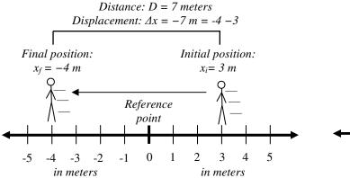
But what if an object turns around? The distance traveled would continue to increase, but the displacement would begin to decrease as the final position became closer to the initial position. If it were to return to its initial position, its displacement would be zero.
